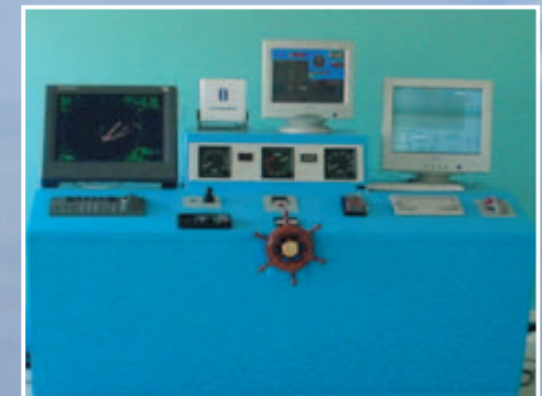
Radar & ECDIS console
